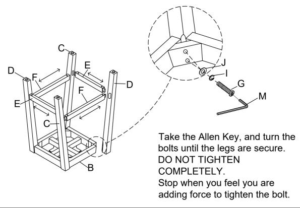
Secure the Front / Rear Stretcher (E) and Side Stretcher (F) with Left Leg (C) & Right Leg (D) using Screw (O) by Screwdriver (P) as below shown.
