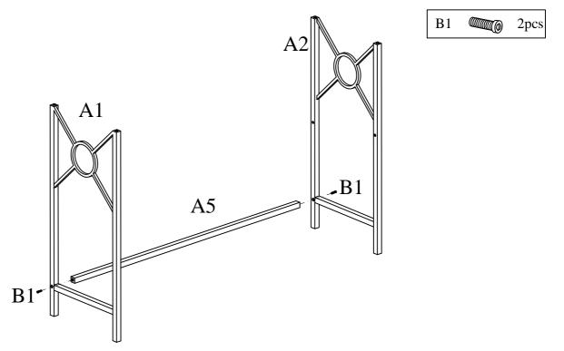
Assemble Connecting Bar A5 to Side Frames A1 & A2 using Bolts B1. Note: Please do not tighten bolts B1 until Step 4.
