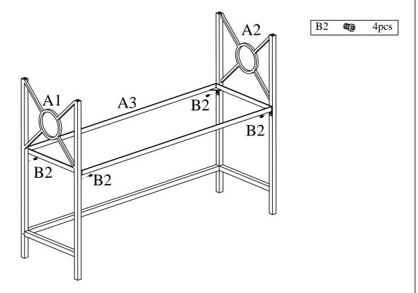
Assemble Middle Frame A3 to Side Frames A1 & A2 using Bolts B2. Note: Please do not tighten bolts B2 until Step 4.
