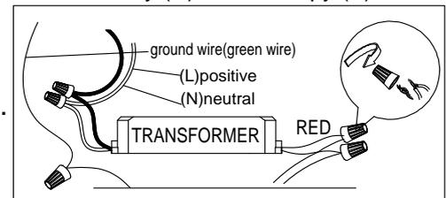
Step.3: Wire fixtures to red wires of the transformer, wire black and white wire of the transformer to wires in outlet box. Silver wire is for ground.
