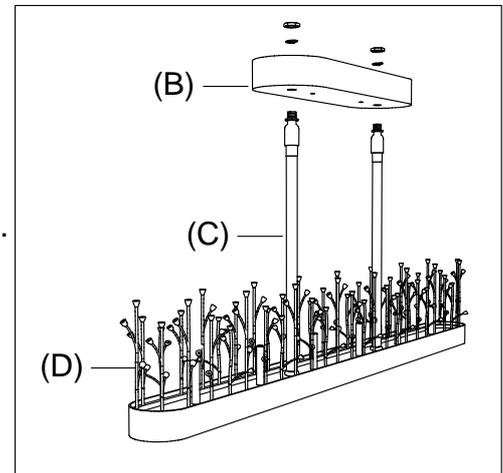
Step.2: Determine correct length of rod needed for hanging height. Screw the Rod (C) on the Body (D) and Canopy (B).
