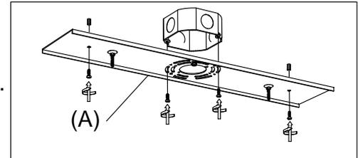
Step.1: Remove Mounting Strap (A) from fixture and install to electrical box.
