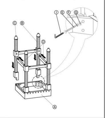
5. Use screws (H) to tighten the stretchers (D) to the leg assembly with Phillips head screwdriver.
