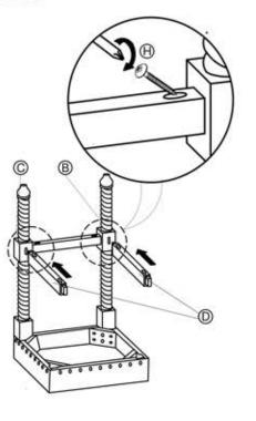
4. Insert second leg assembly to seat frame (A), stretchers (D) as shown. Use bolts (E), spring washer (F), and flat washer (G) to tighten leg assembly to seat frame (A) with Allen key (I).
