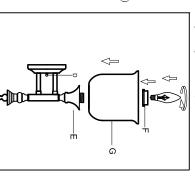
Step.3: Put the glasses (G)with the covers (F) into the cups (E). Use Max 60W bulbs.
