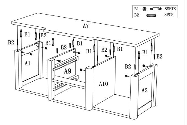
Assemble Top Panel A7 to Left Panel A1, Right Panel A2, Left Divider A9 and Right Divider A10 using Camlocks B1 and Wood Dowels B2.
