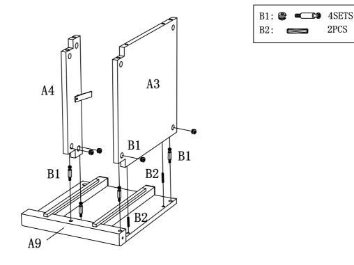
Assemble Middle Shelf A3 & Cross Bar A4 to Left DividerA9 using Camlocks B1 and Wood Dowels B2.
