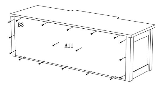
Assemble Back Panel A11 to the back of the unit using Screws B3.
