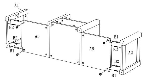
Assemble Side Panels A1 & A2 (L&R) to Shelf A5 & A6 (L&R) using Camlocks B1 and Wood Dowels B2.
