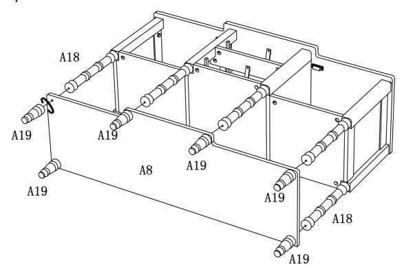
Attach and tighten Bottom Legs A19 by inserting the legs through the Bottom Shelf A8 and attach it to Center Legs A18.
