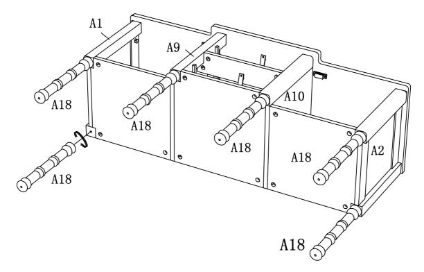
Attach and tighten Center Legs A18 to the bottom of Left Panel A1,Right Panel A2,Left Divider A9 and Right Divider A10 as shown above.
