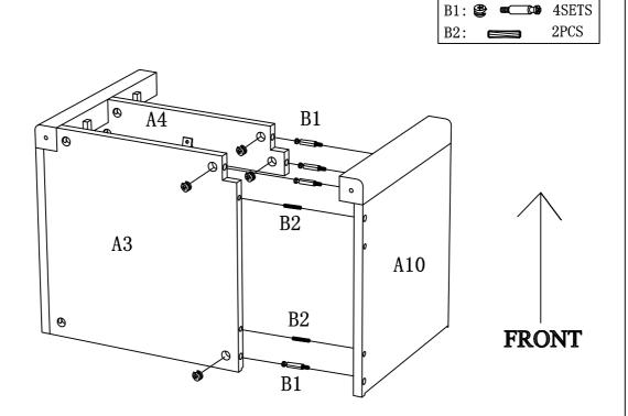
Assemble Middle Shelf A3 & Cross Bar A4 to Right Panel A10 using Camlocks B1 and Wood Dowels B2.
