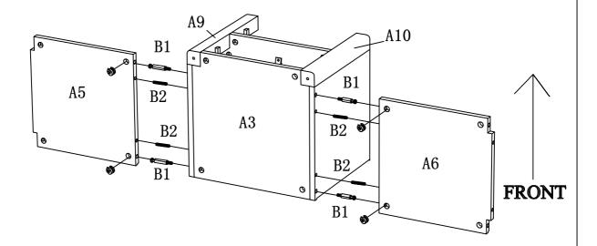
Assemble Shelf A5 & A6 (L&R) to Dividers A9 & A10 (L&R) using Camlocks B1 and Wood Dowels B2.
