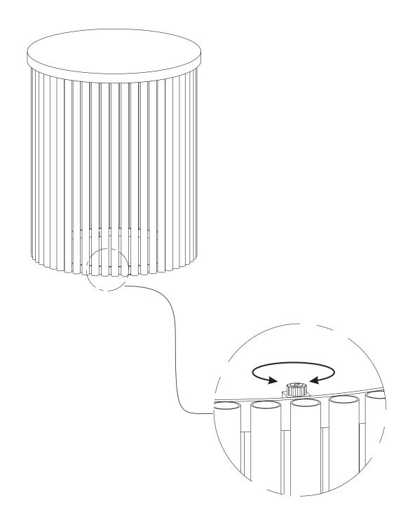
Note: Levelers on bottom of base can be adjusted if floor is uneven.
