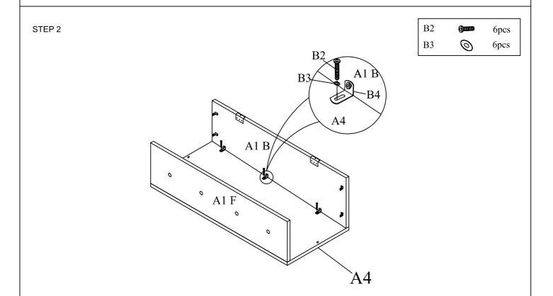
Assemble Back Panel A1(B) and Front Panel A1(F) to Bottom Panel A4 using Bolts B2 and Flat Washers B3.
