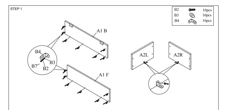
Attach Brackets B4 to Front Panel A(F), Back Panel A1(B), Right Side Panel A2(R) and Left Side Panel A2(L) using Bolts B2, Flat Washers B3. (Please do not tighten Bolts B2 until Step 4). Note: Holes are pre-drilled.
