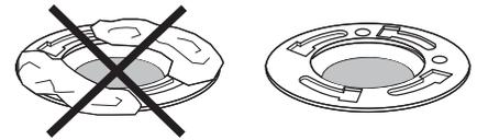
**Caution:** If leaving floor flange open for more than 1-2 hours, cover flange to prevent escaping sewer gases.
