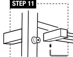
**STEP 11:** Install shelf (k) by inserting the shelf's mounting tube on to the bracket and tighten by inserting the set screw (c) into the hole.
