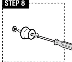
**STEP 8:** Insert long screw (i) through mounting bracket (g), then screw into plastic drywall anchor (f).
