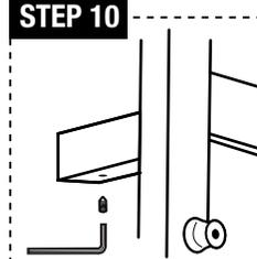
**STEP 10:** As shown in the picture, install the set screws (c) into the hole of all the tubes (a) using the allen wrench; fix the tube (a) onto the mounting bracket (g).
