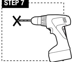
**STEP 7:** Drill A, B, C, and D holes with an appropriately sized bit. Use a hammer to knock plastic drywall anchor (f) into wall completely.
