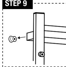
**STEP 9:** Install the tube (a) onto the bracket (g).
