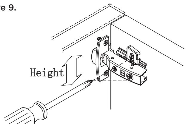
**NOTE:** When adjusting the door hinges keep in mind to adjust the other hinges.
