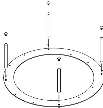
**Step 2:** Carefully lay the vanity on its back and install the metal base.
