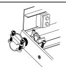
Mount housing to desired surface with the two captive mounting screws (5) provided.
