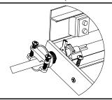
Using wire nuts (provided), attach black fixture wire to black supply wire, white fixture wire to white supply wire, green fixture grounding lead to grounding lead. Unit is TRIAC or ELV dimmable. Follow dimmer manufacturer instructions for proper intsallation.
