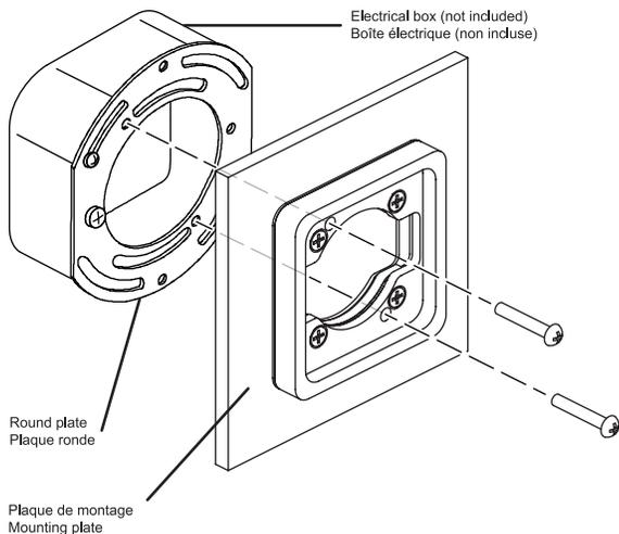
Install the round plate on the junction box, then secure the 4" mounting plate on the round plate and install the mounting bracket on the 4" square plate.
