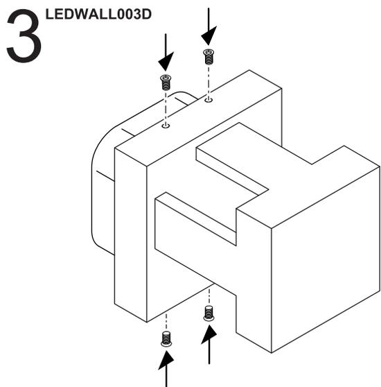
Push all the wires inside the junction box and secure the fixture on the mounting bracket using the 4 set screws.
