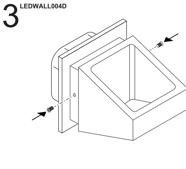
Push all the wires inside the junction box and secure the fixture on the mounting bracket using the 2 set screws.
