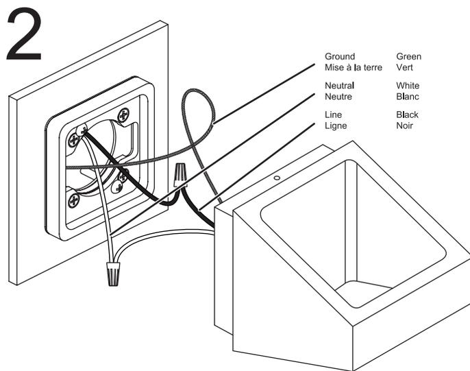
To make the connections in the compartment: use the included wire connectors to match the white wire from the line feed with the white wire from the fixture, repeat with black wire and then connect copper wire (ground) to the green wire.
