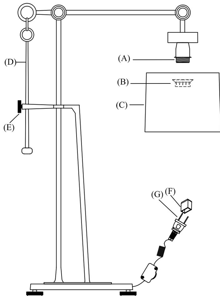
1. Remove socket ring (B) from socket (A).
