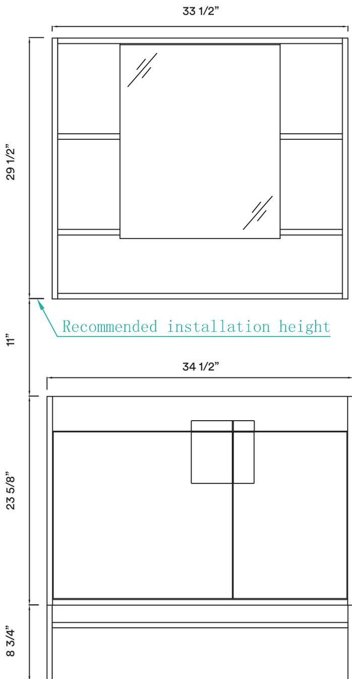
**ATTENTION!** Dimensions may vary by up to 3/8". It is highly recommended to pull all dimensions of actual model for installation and measuring purposes.
