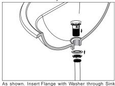
drain Hole. From underside, thread Drain Body into Flange. Holding the drain body in position with Ball Rod Opening facing back, tighten Metal Locknut securely. Thread Drain Tailpiece into Drain body.
