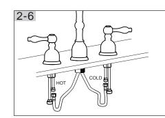
Connect Spout hot water flexible hoses to the Left Valve Side Connector. Tighten flexible hoses Nut. Connect Spout cold water supply line to the right Valve Side Connector.
