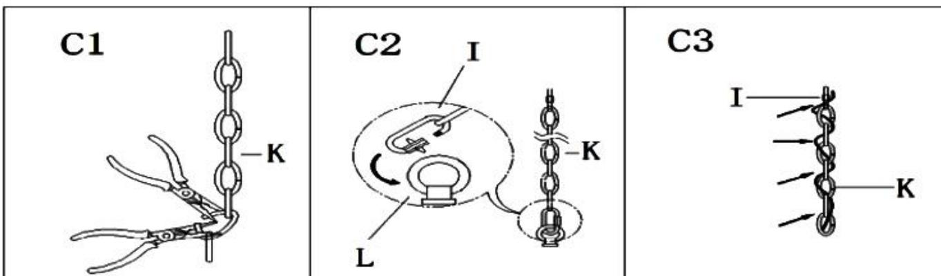
Step C1: By measuring, determine the correct length of links needed. Use the chain pliers, open and discard the remaining chain.
