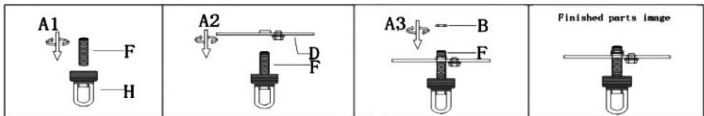
Step A1: Thread the nipple (F) into the screw collar loop (H)
