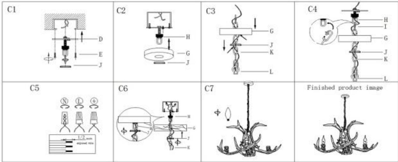
Step C1: Attach single bar (D) to outlet box with mounting screws (E). The side of single bar marked "GND" must face out
