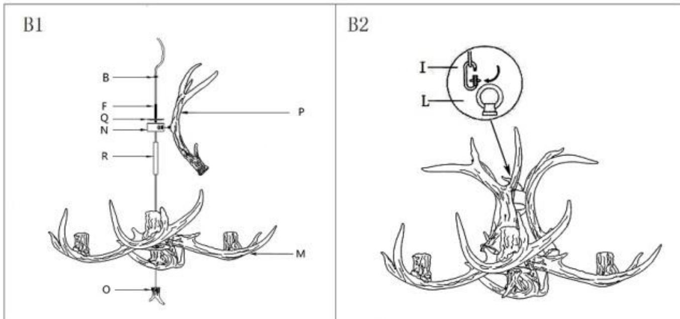
Step B1: Unscrew the ball nuts(N), hex nut(B) from the antler(P).
