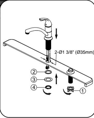
For models with spray: Insert spray support through far right hole on sink. Screw hold - down nut (1) onto shank and hand tighten. Place faucet in position on sink. Install rubber washer (2) and metal washer (3) onto the threaded mounting shank. Thread nut (4) onto mounting shank. Do not overtighten.
