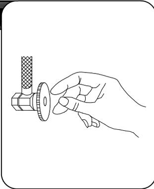
Shut off water supply at angle stop. Clean sink surface in preparation for new faucet. If your model has a spray, proceed to step 2. If your model does not have a spray skip to step 4.
