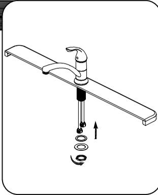
Place faucet in position on sink. From underneath sink, install rubber washer (1) and metal washer (2) onto the threaded mounting shank. Thread nut (3) onto mounting shank. Do not overtighten.
