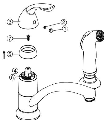
Shut off water supply. Remove set screw plug (1). With valves in "closed" position, unscrew set screw (2) and remove handle (3) from valve stem (4). Loosen the screw (7) from valve stem (4). Loosen the cap (5) from the sleeve (6).
