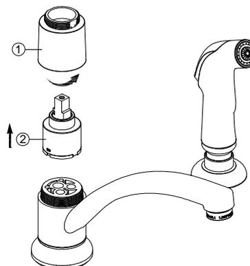
Loosen sleeve (1) by turning it counter-clockwise and lift out the cartridge (2). Remove the old cartridge and replace with the new cartridge. Replace sleeve and tighten. Reinstall the handle.
