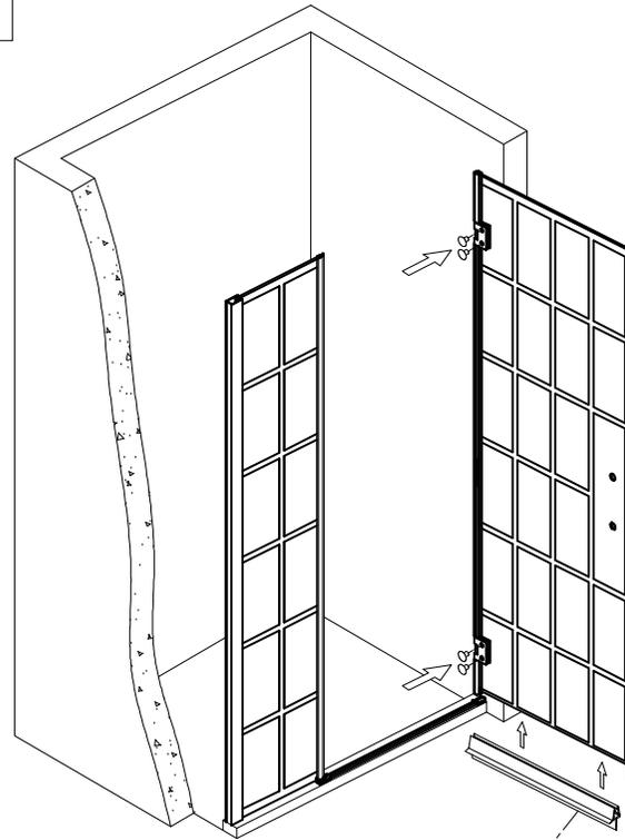
IT IS VERY IMPORTANT TO HAVE THE BOTTOM OF THE GLASS PARALLEL TO THE TRAY TOP FACE, IT MUST HAVE A 22mm EVEN GAP ALL THE WAYALONG.
