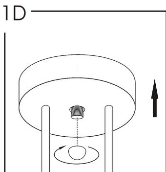
Lining up threads on crossbar with hole in backplate, attach fixture to junction box using cap nut. Be sure to carefully tuck wires into backplate while attaching.
