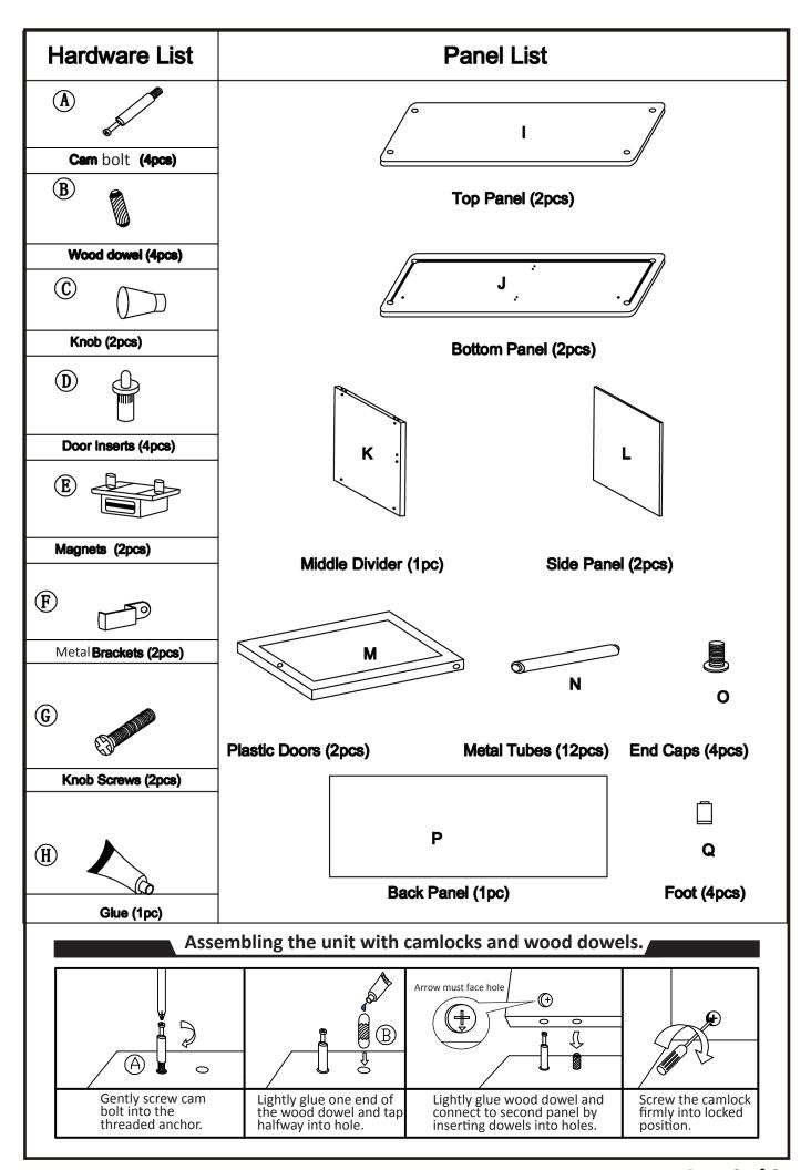
(1) Place bottom panel (J) with groove side up on top of the four black plastic feet (Q).
