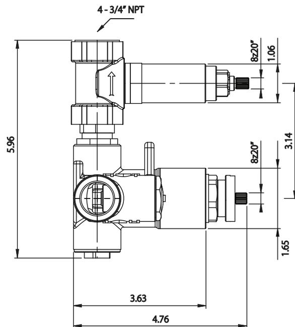
TVH.4101 | 3/4" Thermostatic Valve With Volume Control Page 2 of 2
