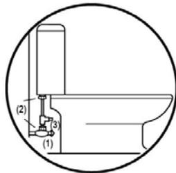
Shut water supply by turning it to the right and disassemble the water hose.
