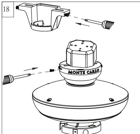
18 Install 2 of the screws to the side panel of mounting bracket corresponding to the open slotted holes on the canopy upper rim, screws provided. Remove the thread studs from the lower part of the mounting bracket.
