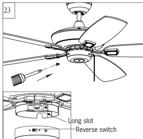
23 Align the long slot on top plate with the reverse switch on switch housing, and then install the switch housing onto the top plate with the 3 set screws removed in step 21 and tighten all screws securely.
