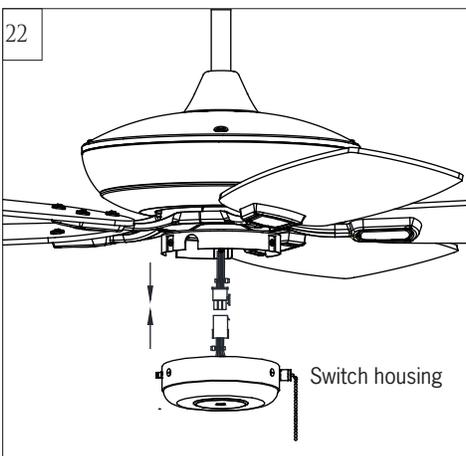
22 Connect the plug from fan with the plug from switch housing. Be sure plugs connection clasped together completely.
