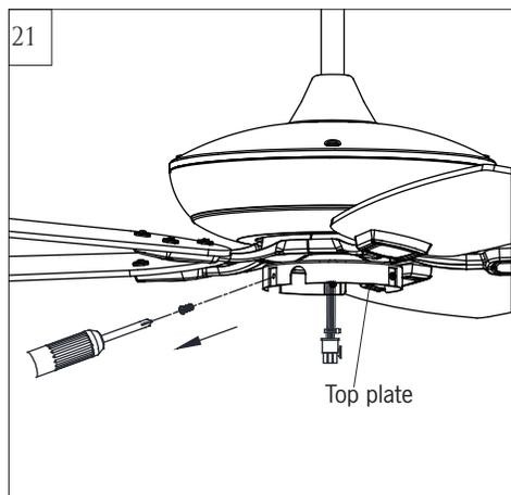
21 Remove the 3 set screws on top plate of switch housing, keep screws.
