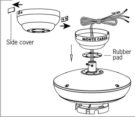
Remove side covers from canopy exposing 4 holes. 2 closed holes and 2 open "L" shape holes. Place rubber pad and canopy over lead wire and safety cable and align the larger holes in canopy and holes on rubber pad with the set screws on yoke.
