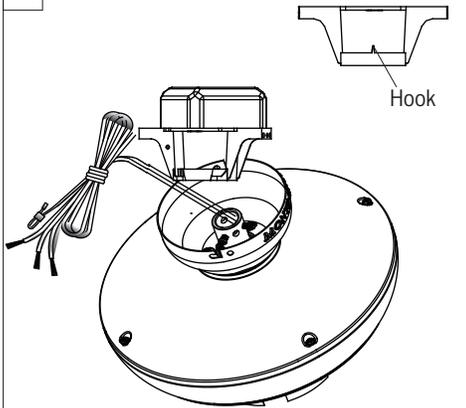
To prepare the fan for wiring, hang fan onto mounting bracket by sliding the canopy over the mounting bracket hook **(Use one of non-slotted holes on the rim of the canopy)**.
