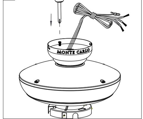
Reinstall the 3 set screws remove in step 12. Tighten screws securely.
