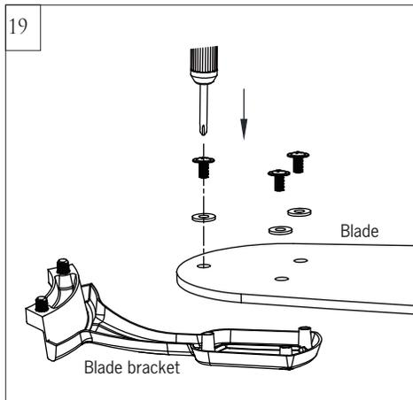
19 Install blade bracket with blade by 3 blade screws and washers provided. Tighten screws securely. Repeat this process for remaining blades.
