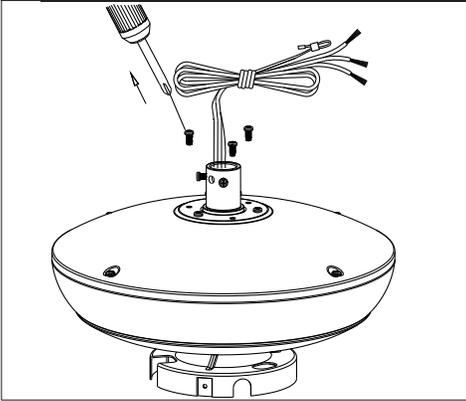
Remove every other screws from yoke located on top of fan assembly. Keep screws.
