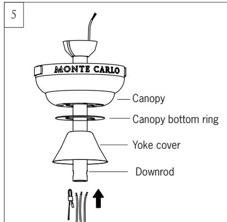
Place downrod over canopy, canopy bottom ring and yoke cover. Thread lead wires and safety cable from motor assembly through downrod.
