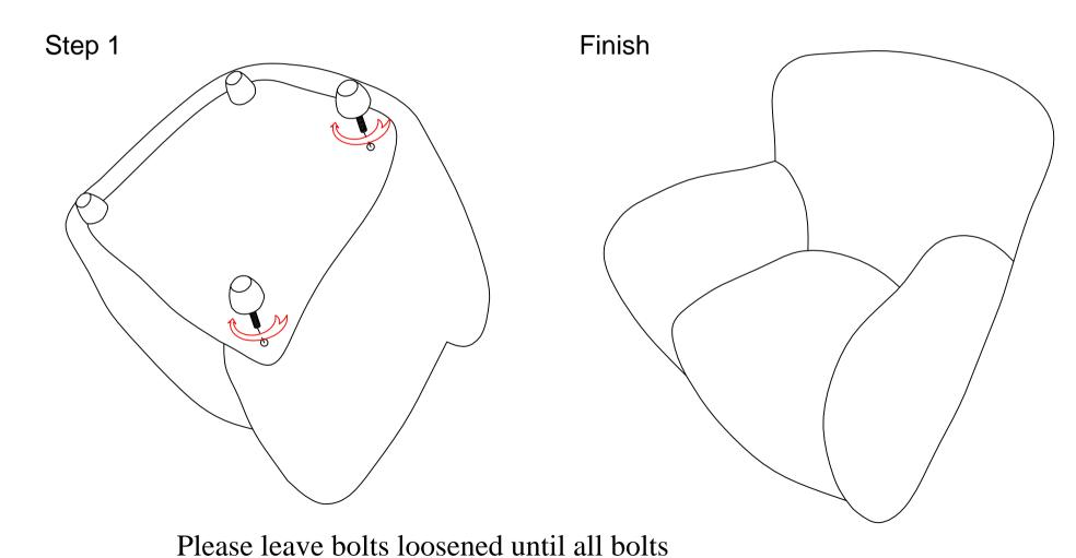
are placed before tightening completely
