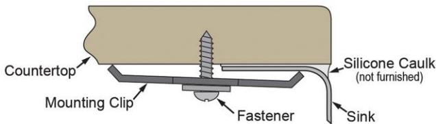
Designed to affix to the underside of any solid surface countertop.
