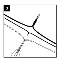
4. Attach wire nuts (BB). Tape wire nuts (BB) and wires together.
