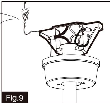
Hang the safety cable into the safety cable hook, tighten the safety cable to the safety cable hook by using the zip-tie.
