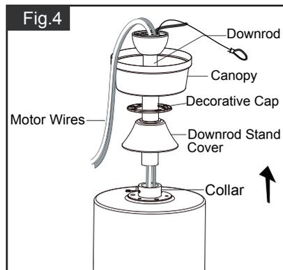
Thread the motor wires through the downrod stand cover, decorative cap (Making sure the smooth side of decorative cap is facing downward.), canopy and downrod.
