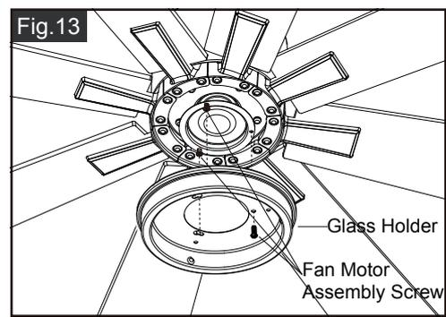
Remove one fan motor assembly screw (for later use), push the glass holder upwards until the fan motor assembly screws insert into the key hole slot of glass holder then rotate the glass holder till it is fixed on the motor bottom. Finally, secure the glass holder to motor bottom with previous screw which we removed and tighten the other two fan motor assembly screws.
