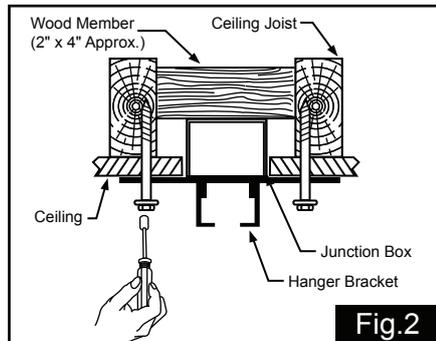
Tighten the hanger bracket to the outlet box with two mounting screws. **(Make sure the outlet box is securely installed so that it will be able to support at least the fan weight.)** Attach the safety cable hook to the ceiling and make sure the safety cable hook is covered by the fan canopy.
