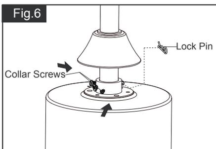
Tighten the two collar screws. Slide lock pin into hanger pin until it is locked into position.
