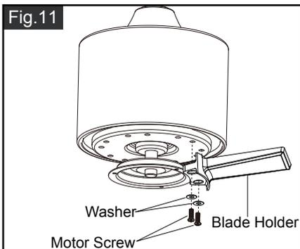
Remove the motor screws and washers from the motor assembly. Secure blade holders to the motor with washers and motor screws.
