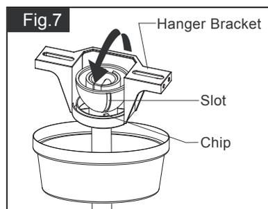
Hang the fan on hanger bracket, and make sure the slot of hanger ball is snapped into the chip of hanger bracket exactly. **Note: For sloped ceiling installation, make sure the slot of hanger ball and the chip of hanger bracket face down.**
