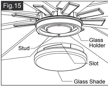
Attach the glass shade to the glass holder by aligning studs and slots, and then turn it clockwise until it is locked in place.
