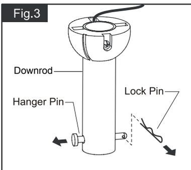
Remove the lock pin from the hanger pin and remove the hanger pin from the downrod.
