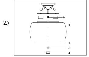
Step 2. Place glass(E) over Nipples (D), and secured with Metal Plate (H) and Hex nut(I), attach Finial(K).
