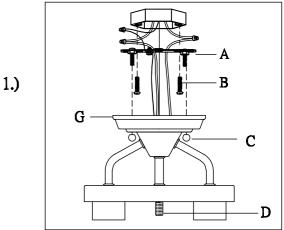
Step.1: Install the Crossbar (A) to electrical box by Screws (B).
