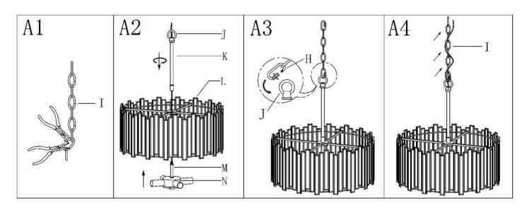
Step A1 » By measuring, determine the correct number of links needed for proper hanging height. Using the chain pliers, disconnect and discard the unwanted part.
