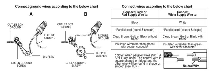
Twist wires together with plastic wire connectors until tightly joined.
