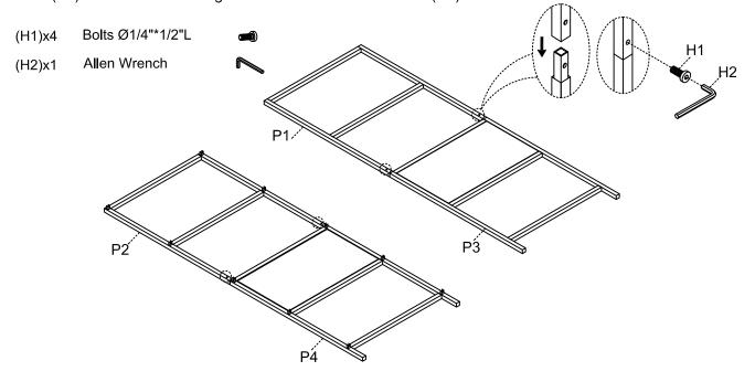
**Step 2.** Attach the assembled side frames (P1,P2,P3,P4) to the shelves (P5) and center panel (P6) as shown below.
