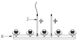
Gently pass wires through the hole of bars on frame(I) and then put the frame(I) onto the stems (J)
