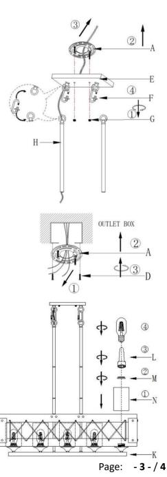
5. Unscrew the knob nuts (G)from canopy (E) then remove the mounting plate (A)
