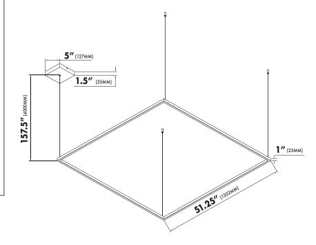
THE MEASUREMENTS ARE ROUNDED TO THE NEAREST  $1/4^{\prime\prime}$
