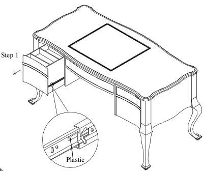
Press the left side plastic up, and press the right side plastic down, then pull out the drawer.
