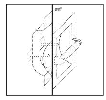
Tighten the screws until the clamp is firmly secured against the inside of the wall.
