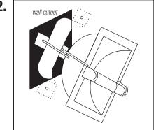
Angle the clamp through the hole by first tilting it to one side, and then the other. Be careful not to damage the wall board.
