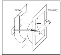
Attach the clamp to the accessory by inserting the screws through the accesory into the bracket. Turn screws three full turns.
