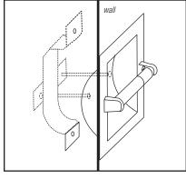
Position the accessory squarely with the flange (outer edge) pressed firmly against the wall.
