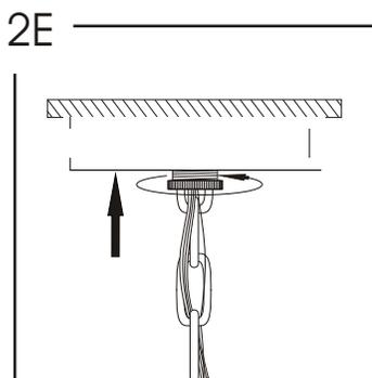
Carefully tuck wires into junction box and secure canopy to ceiling using screw collar ring.
