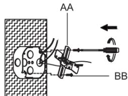
3. Strip 3/4 in. of insulation from fixture wire ends. Twist stripped ends together with pliers (not included), black to black (power), white to white (neutral). Snip ends. Wrap the ground wire from the outlet box around the green screw preassembled on the cross bar (AA), and then connect the ground wire from the outlet box to the ground wire from the fixture.
