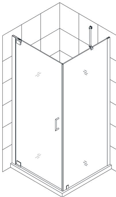
42. Locate the **Support bar (22)**. Position the bar on the stationary glass at a 45-degree angle between the glass and the wall if possible. Level it horizontally. Hold it firmly in place and outline the bracket's position on the wall. Remove the **Support bar** and detach the wall bracket from it using the supplied Allen wrench. Place the wall bracket against the outlined position on the wall and mark the hole for drilling. (Fig 45.3)
