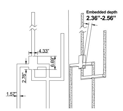
2. install main body inlet and outlet pipes.
