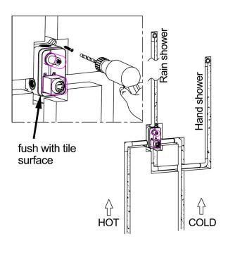
3. Fix ceramic tiles, cut off the edges of the embedded box, remove the protective cover and install the panel.
