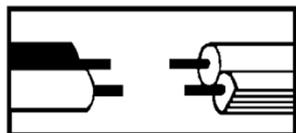
\*Note: When parallel wire ( SPT I & SPT II ) is used. The neutral wire is square shaped and ridged and the hot wire will be round in shape and smooth. ( See Illustration on left. )
