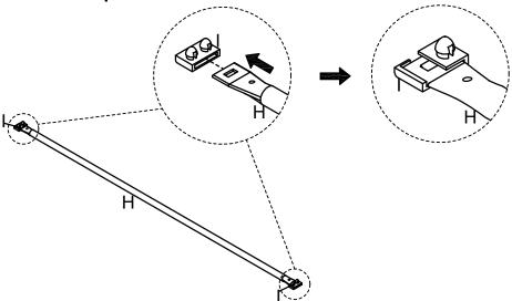
Attached the Slat (H) to rails, put the Slat Connectors (I) into the correct place and press them down.
