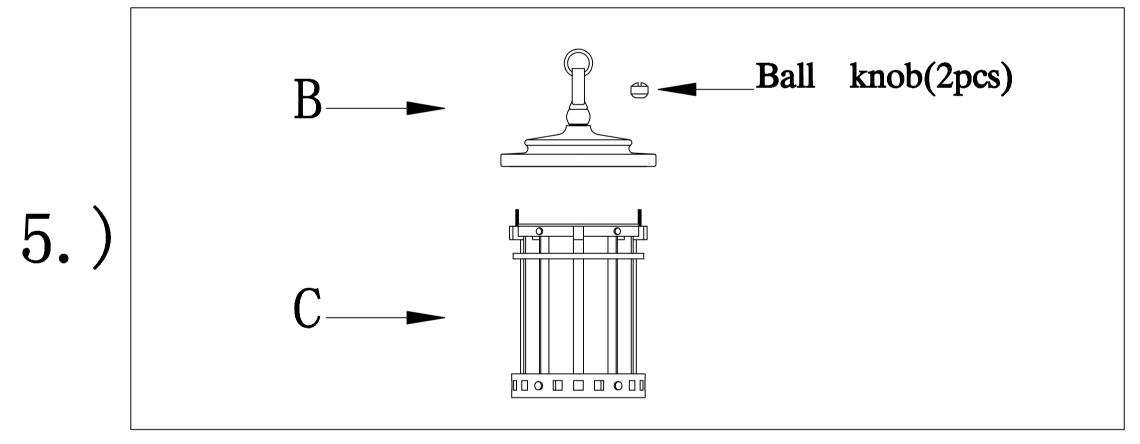
Step.5: Attach cage(C) to fixture, using ball knobs.
