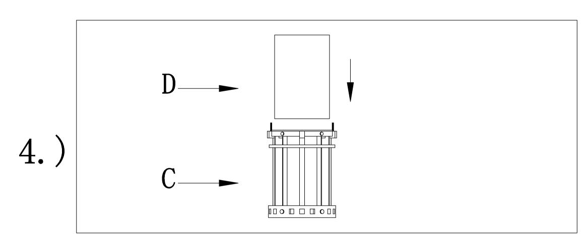
Step.4:Install the glass shade(D) into the cage(C)
