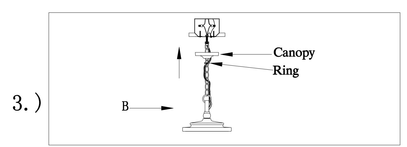
Step.3: Remove ring from loop and slide down chain. Place canopy onto chain and let slide to top of fixture. Install screw collar loop to bracket. Pull canopy through screw ring up chain to ceiling and tighten securely.
