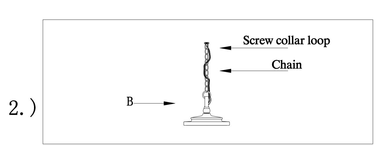
Step.2: Install chain to fixture(B), install screw collar loop to chain. Attach appropriate amount of chain to loop to achieve desired mounting height. Thread wire through every 3rd loop of chain.
