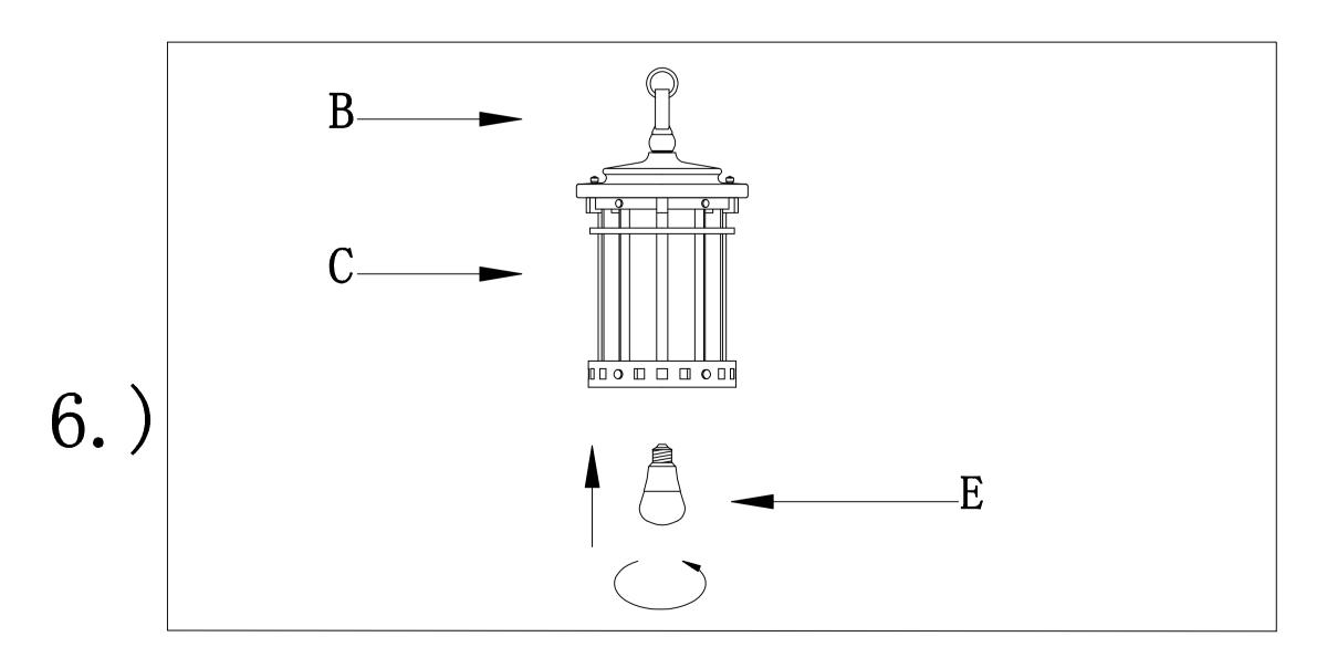
Step.6: Install E26 LED bulb(E)
