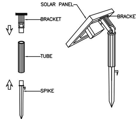
5. INSERT THE SPIKE INTO THE GROUND. POSITION THE SOLAR PANEL TO FACE SOUTH (In Northern Hemisphere) AS MUCH AS POSSIBLE TO MAKE THE MOST OF THE DAYLIGHT HOURS. IT IS IMPORTANT TO ANGLE THE SOLAR PANEL TO FACE SUN WHEN SUN IS AT ITS HIGHEST POINT. ENSURE THE SOLAR PANEL IS NOT SHADED BY TREES, SHRUBS OR BUILDINGS
