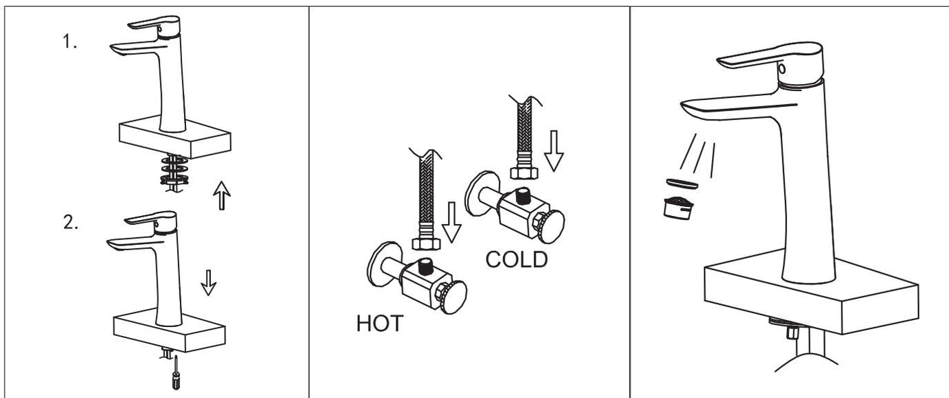
4. Re-install the rubber washer followed by the metal washer and lock-screw. Using the wrench to tighten lockscrews.
