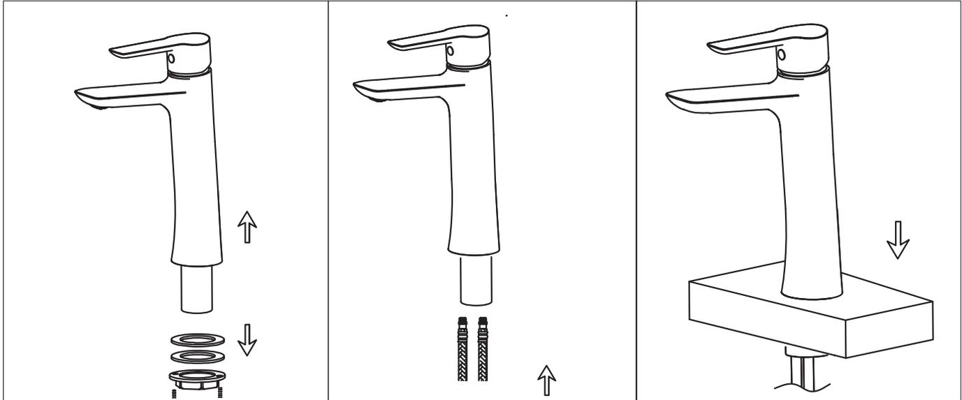
1. Remove the rubber washer, metal washer and locking screw from the faucet.
