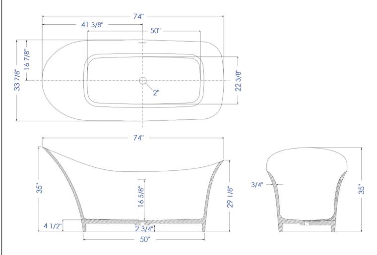
Please Note; Due to thermal expansion and contraction, the total dimension of the tub will have +-2% error, these dimensions are for reference only.
