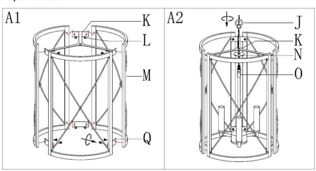
Step A1 » Thread screws (L) into flat iron stent (K), flat iron bars (Q) and iron frame (M) as shown in the illustration.
