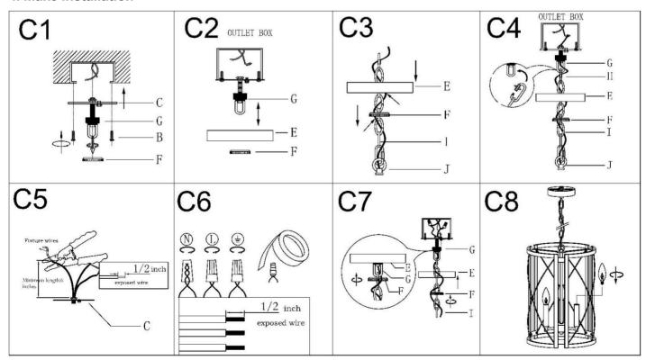
Step C1 » Remove collar ring (F) from collar loop (G). Attach single bar (C) to the outlet box with mounting screws (B).
