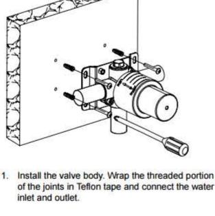
of the joints in Teflon tape and connect the water
