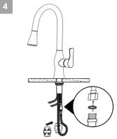
Connect pullout hose to quick connect and insert weight (looseinstall)
