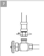
Connect hot and cold water lines to the inlet pipe and tighten with a wrench until snug. Do not over tight.
