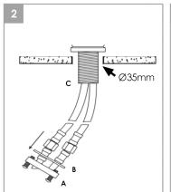
Ensure there is a Ø35mm through-hole on the kitchen counter. Remove the mounting nut (A) and washer (B) from the threaded shroud (C).
