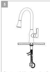
Secure weight on lowest vertical point on pull-out hose side. (not on quick connect side)
