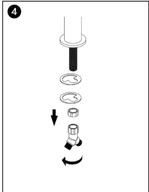
Loosen the fixing nut, washers, and adapter from the body and put aside.
