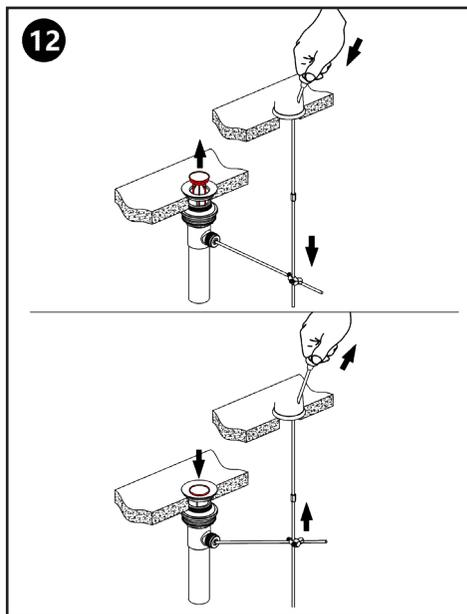
Once connected, to open the drain, push down. To close the drain, pull up. Fill your sink to check for any leaks and to ensure that the drain is functioning properly.
