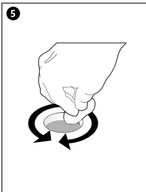
Clear area before inserting pop-up drain stopper.
