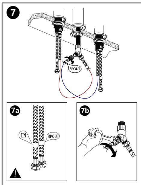
Secure the spout hose lines from the hot and cold water fixtures.
