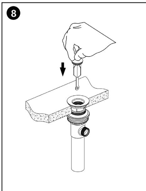
Insert the stopper tailpiece from above. Position the tailpiece hole to align with the hole to the side of the body.
