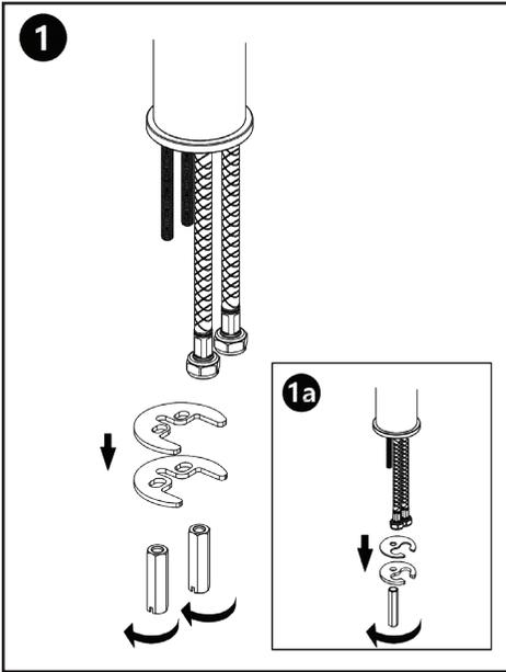
Loosen the fixing nut and screws for the handles and put aside.
