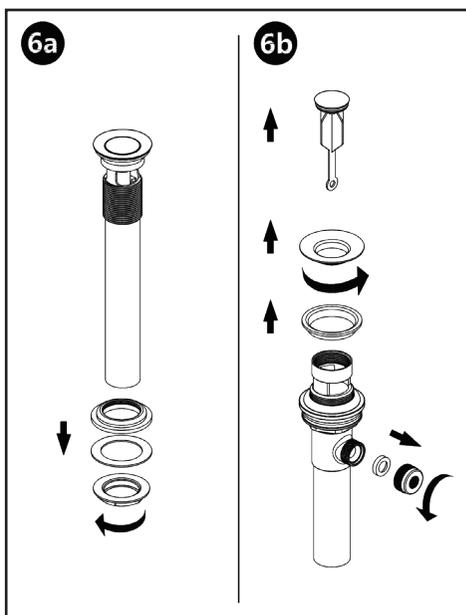
Remove the washer, flat washer, and nut from the pop-up.
