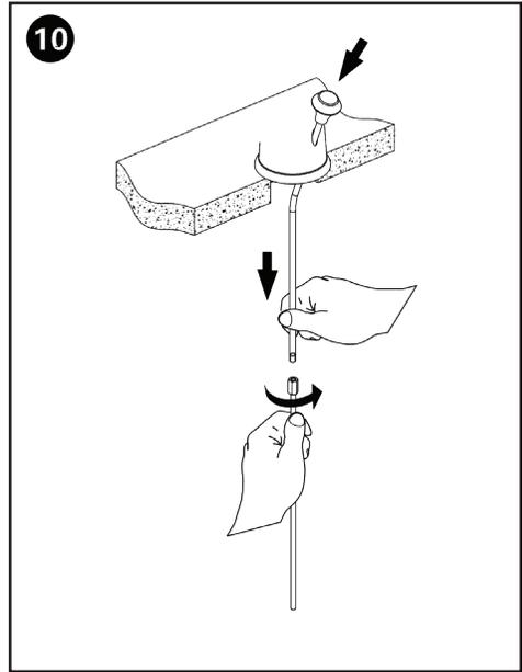
If not already installed, insert the faucet's lift rod into its designated hole on the back of the faucet. Attach the extension rod.
