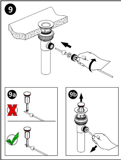
Connect the drain lever by threading it into the hole on the side of the body. The lever must pass through the hole in the stopper tailpiece to function properly.
