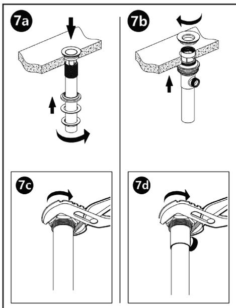
Insert the pop-up from above and tighten the nut and washers below to secure to the counter top.
