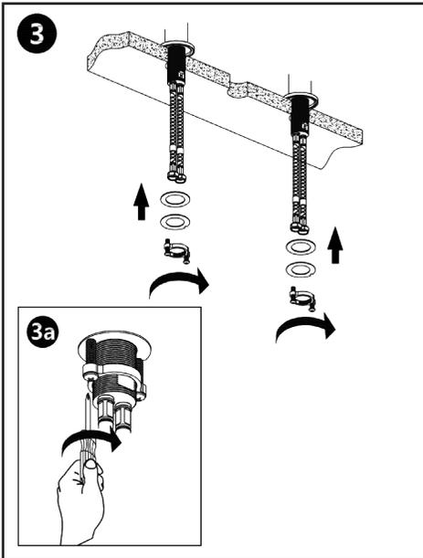
Secure the hardware into place with the Base O-ring, nuts, and screws.
