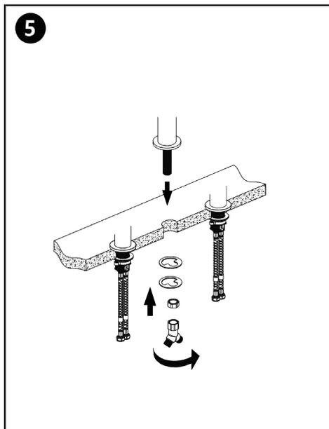
Insert the body into the counter top from above and secure with nuts and washer from below.
