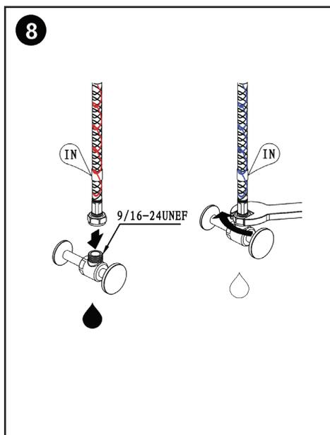
Secure the hoses to the hot (red) and cold (blue) lines appropriately.
