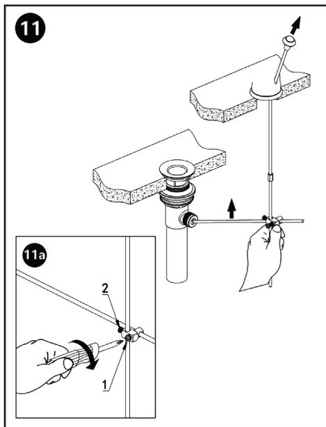
Connect the lift rod and the drain lever with the included attaching clip. Use a screwdriver to secure but do not overtighten the link.
